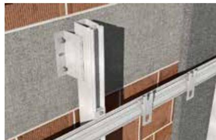
Detail: FPH fixing on concrete
