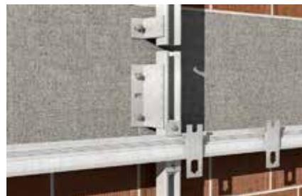
Detail: SPH fixing on concrete
